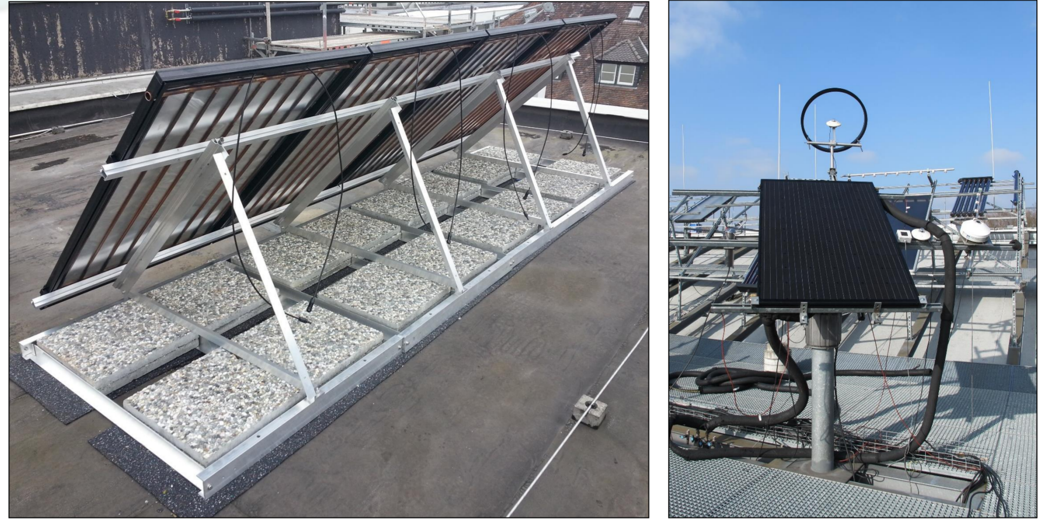
Illustration 3: Image of the PVT collectors on top of the field test building (left) and a PVT collector on the laboratory roof for test measurements and characterization.
