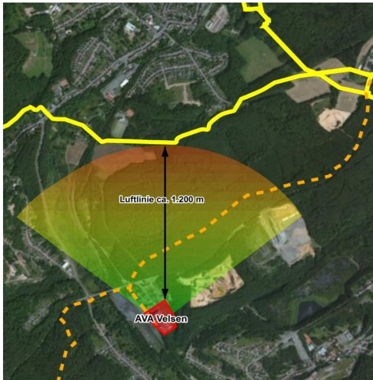
Figure 4: Location of the site of the AVA Velsen to gas networks (mine gas: dashed; natural gas: yellow)
