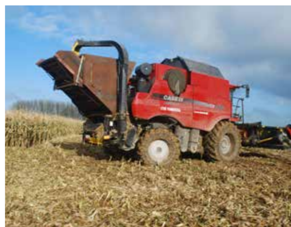
Figure 20: Adapted combine for spindle and husk collection in the bunker at the rear of the combine
