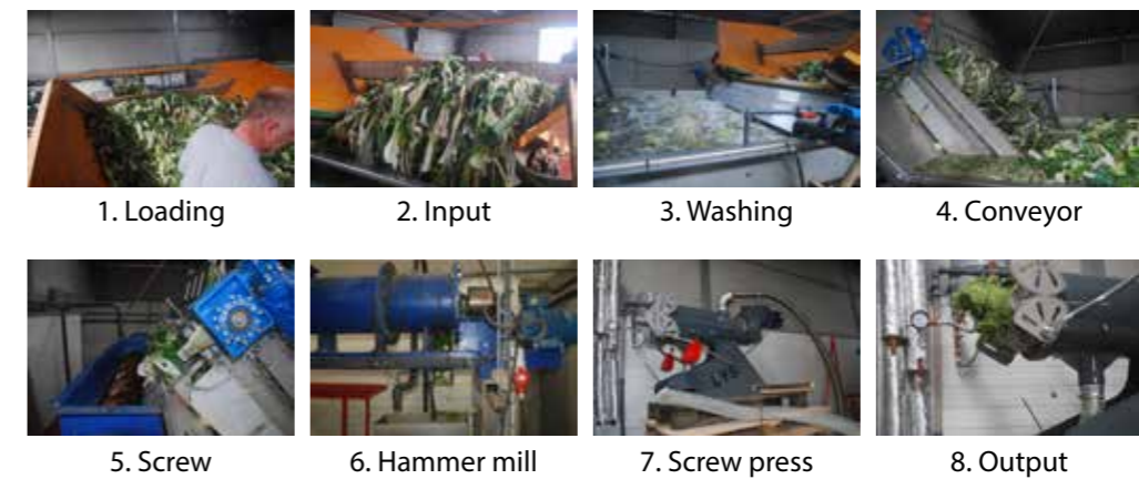
Figure 47: Washing, chopping & pressing experiment with leek residues
