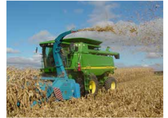
Figure 30: Adapted combine with cutter head to collect and chop stem and leaves (Shinners et al. , 2009)
