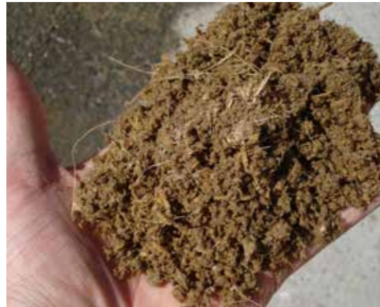
Figure 44: Corn spindles and sprout stems product after hammer mill
