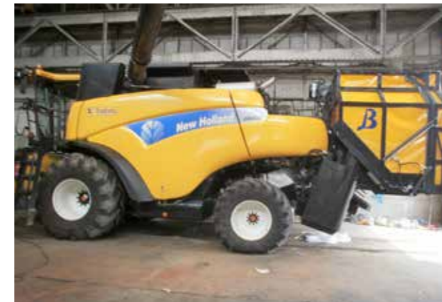
Figure 21: Adapted combine for spindle and husk collection in the bunker at the rear of the chopper
