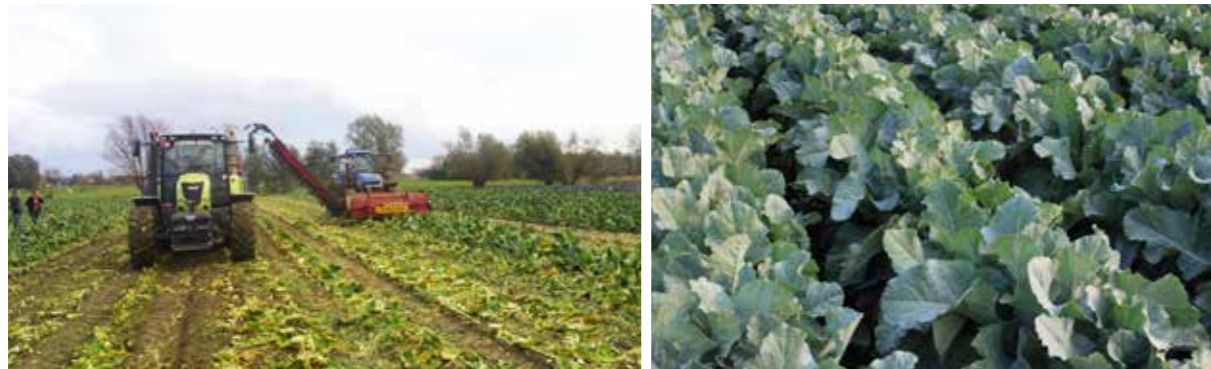
Figure 40: Adapted beet defoliator for the collection of cauliflower residues.
