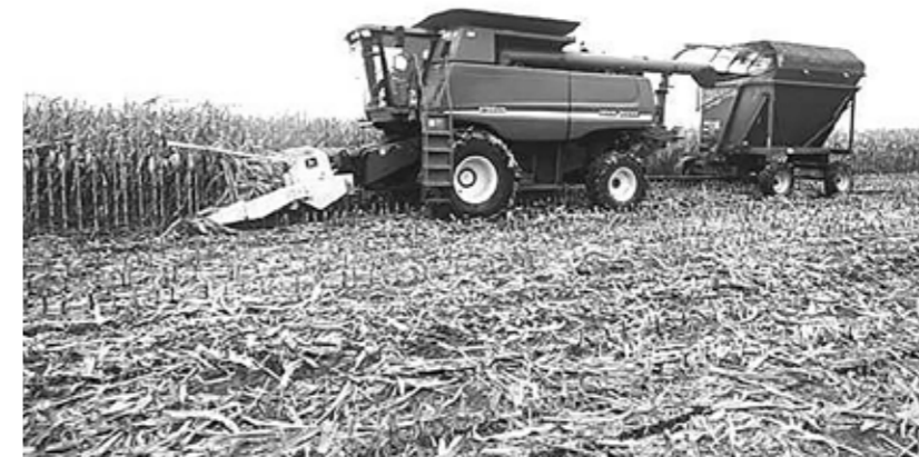
Figure 26: Combine with adapted cutter head to collect all the biomass (Shinners et al., 2009)
