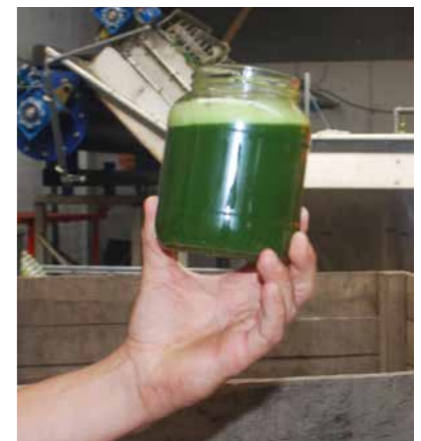
Figure 49: Liquid fraction after pressing of leek residues.
