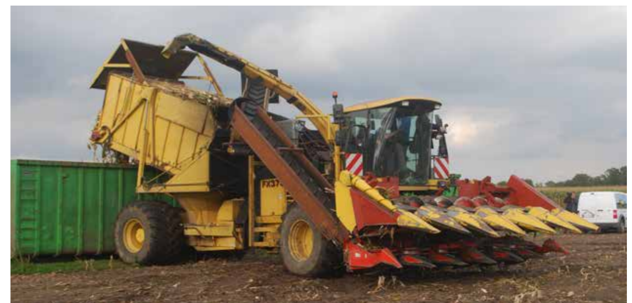
Figure 23: Side view of the adapted combine with two headers by Renders and Kenis
