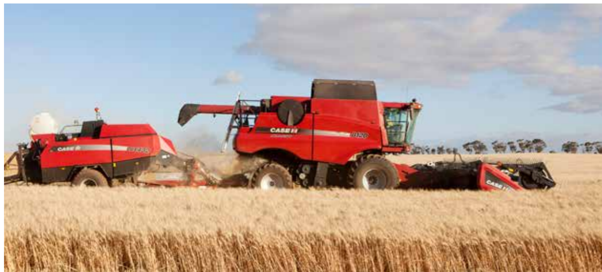
Figure 28: The combine pulling a baler (Verhaeghe, 2013)
