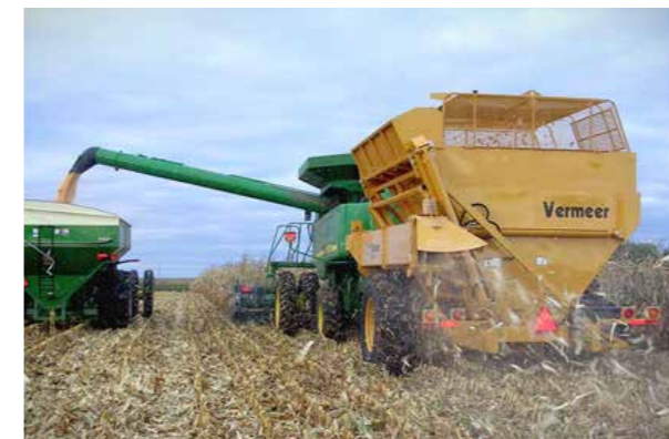
Figure 31: Collection cart with separation of cob and husks (Vermeer, 2009)
