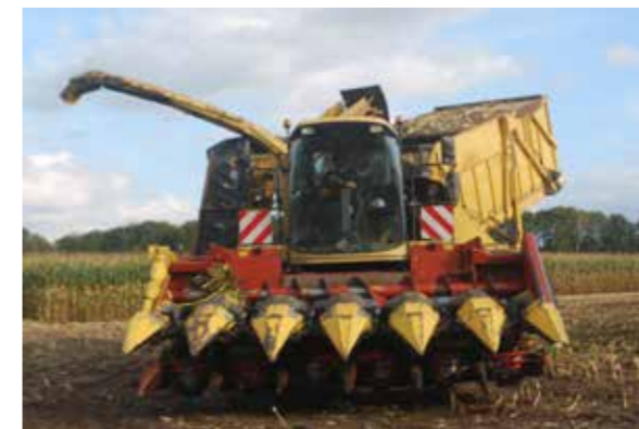
Figure 22: Front view of the adapted combine with two headers by Renders and Kenis
