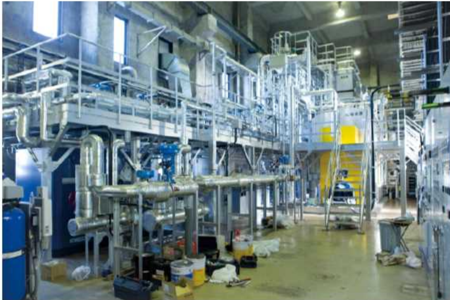
Figure 1: Heat pump-based sewage sludge drying system
